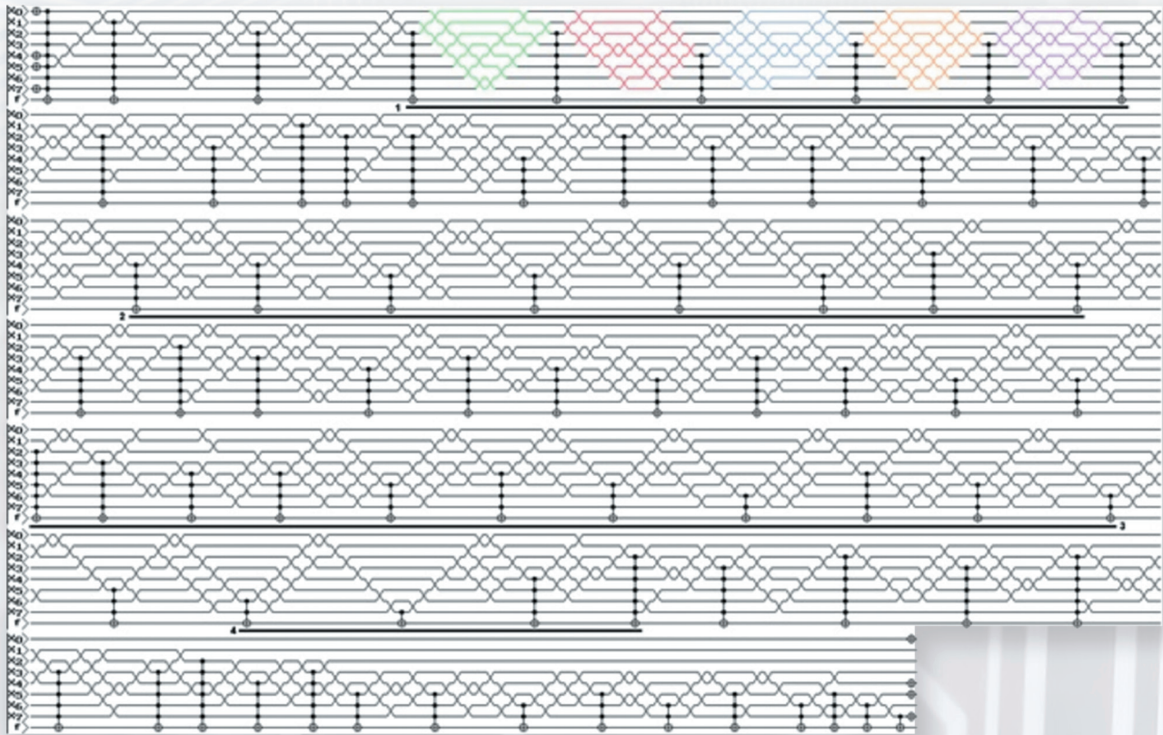
Fig. 5. Direct arrangement of SWAP gates according to FPRM for 141 polarity
